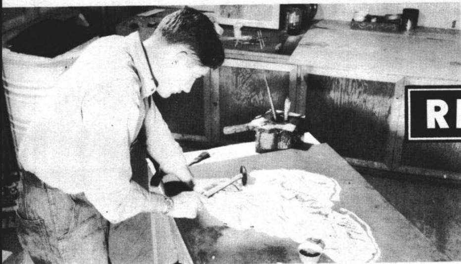
ELEVATION is shown by layers of heavy cardboard (above), which are secured with rubber cement, tacked for rigidity. Landscape details are added (below).
