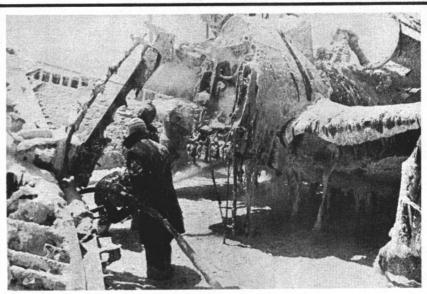
SNOWY bubbles of fog-foam blanket a plane in test of new high-capacity fire-fighting equipment being installed by the Navy on aircraft carriers.
