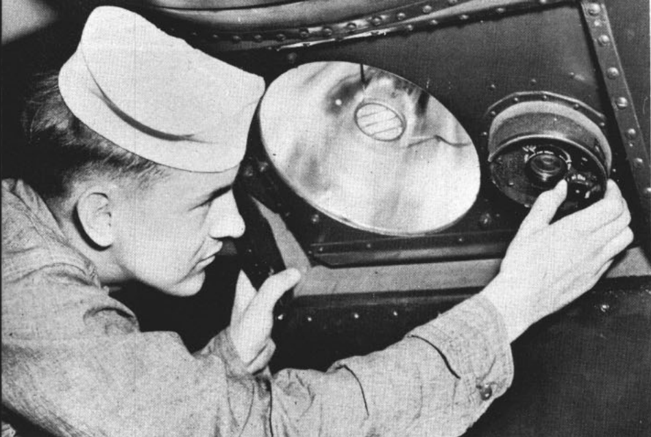
PHOTOGRAPHER'S MATE adjusts aperture of a plane camera prior to takeoff. Camera and synchronized flash tube records antisubmarine operations of TBM3.
