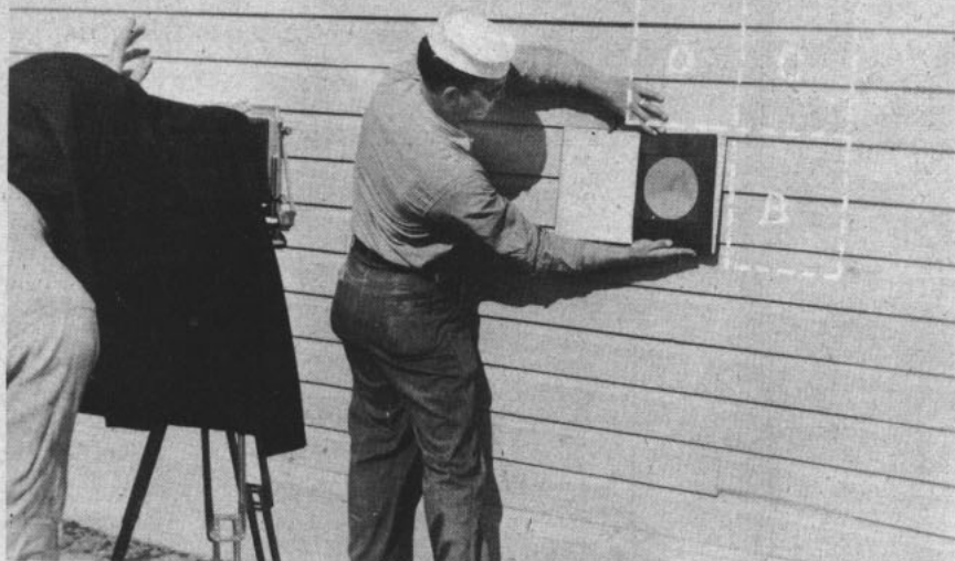
FOUR-IN-ONE photography, this might be called. By placing copy in positions shown, photographer can take four exposures on one piece of film, save money.
