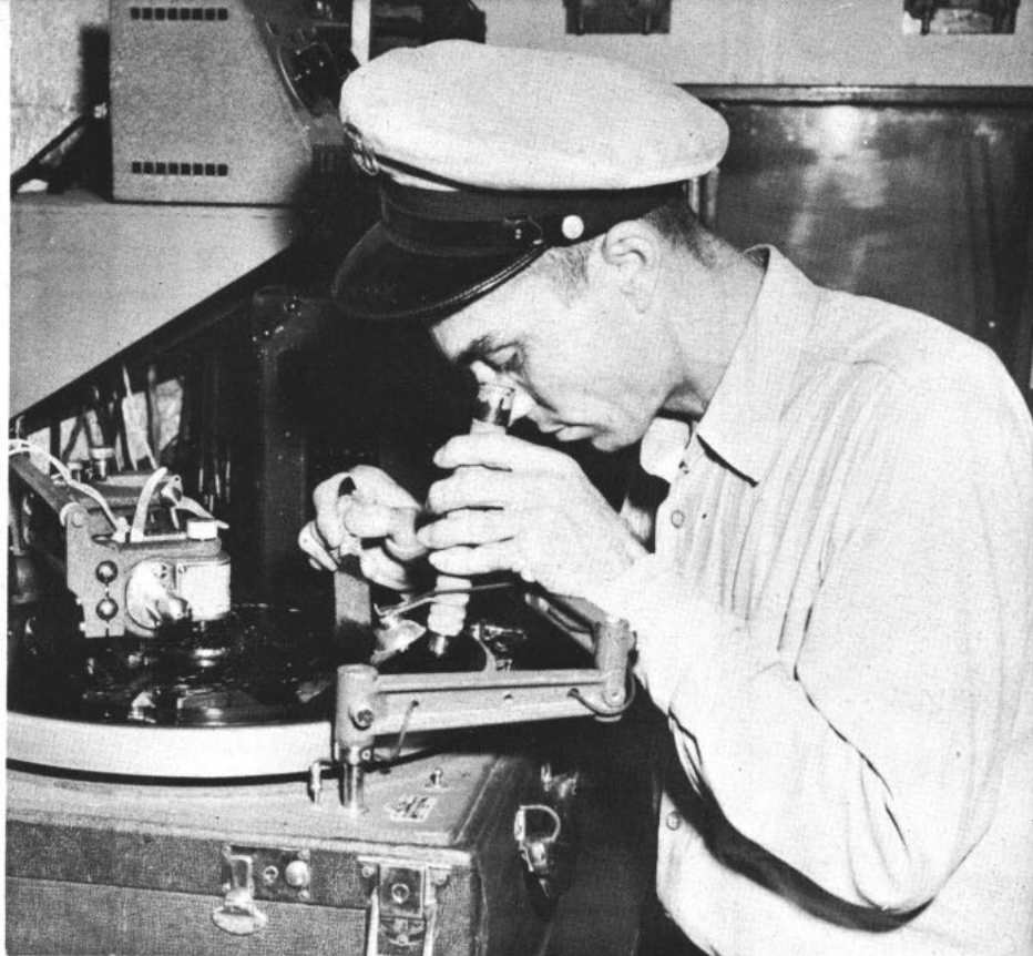
CHIEF in recording laboratory (above) cuts platter used in teaching sonarmen to recognize underwater sounds, while new antisubmarine ordnance (below) gets check on Key West school ship. School squadron often gets first crack at gear.
