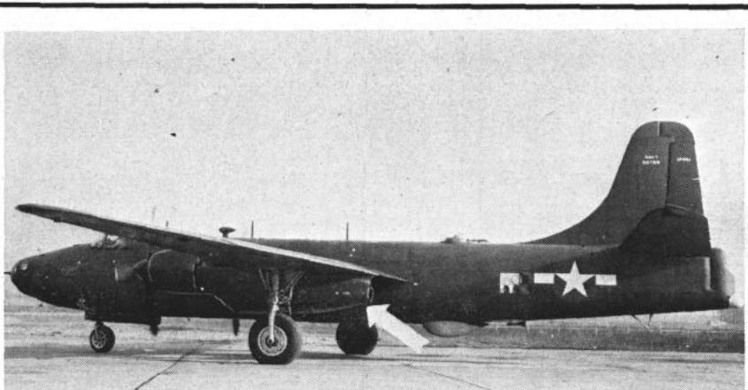
XP4M-1 is powered by two huge conventional engines and two jet engines in two nacelles. Arrow points to jet engine mounted behind conventional engine.
