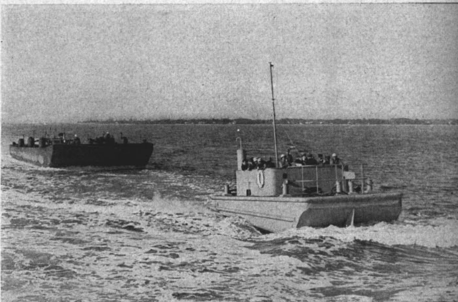
HANDY as a shirt pocket was the diesel or gas-powered YTL—harbor tug, little, shown here towing a barge. Below is a YR—non-self-propelled workshop.
