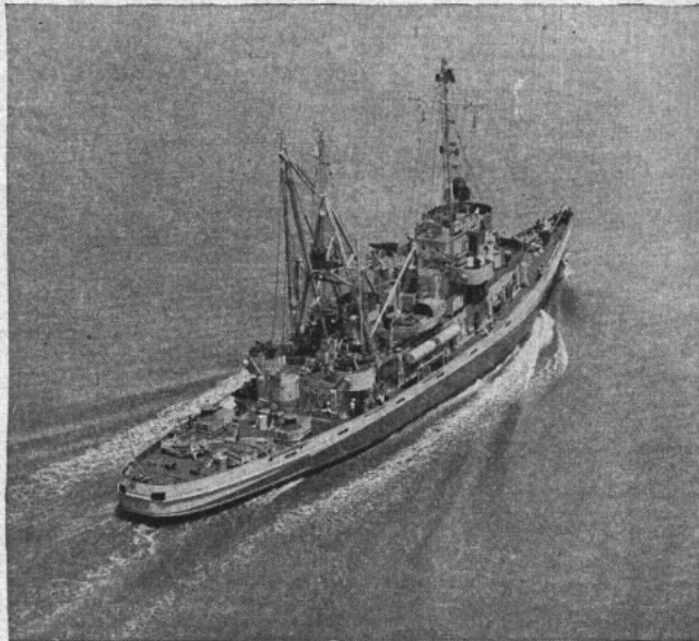
HARD AT WORK , the YTB (at left) demonstrates her adaptability, pushing a gate vessel to unlatch a harbor. The ASR 12 (right) is a submarine rescue craft designed to extricate men from disabled submarines down to 300 feet.
