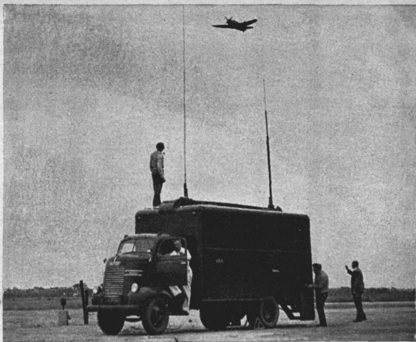
Official U. S. Navy photograph INVISIBLE LINK between Helldiver and recording truck on ground is new telemetering equipment which automatically transmits flight data.
