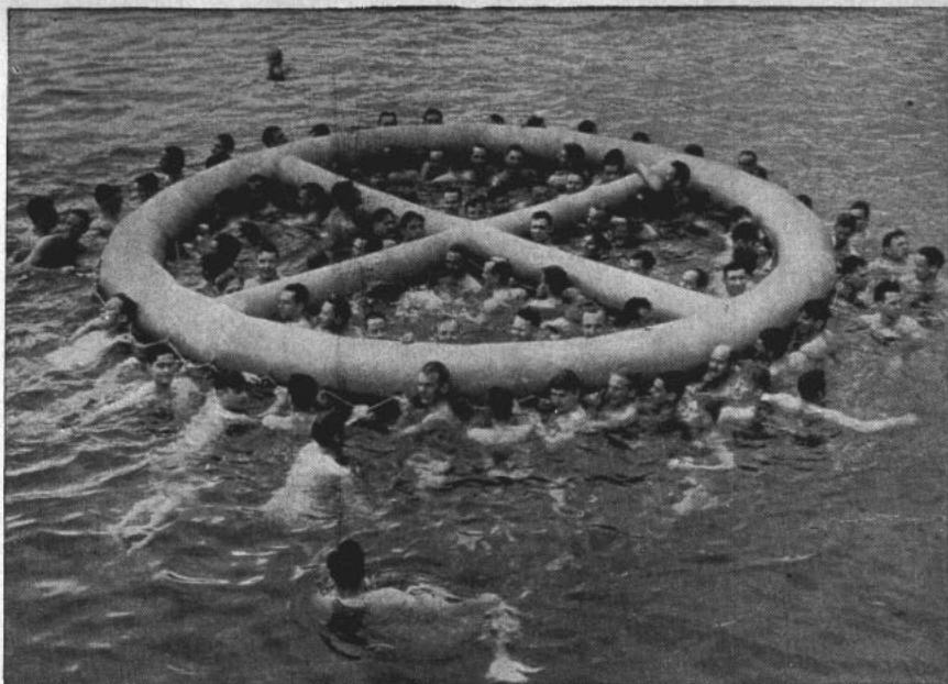
RUB-A-DUB-DUB (REVISED) — Life raft, shown being tested at Wright Field, will accommodate 104 men. Raft is 38 ft. across but weighs only 79 lbs.
