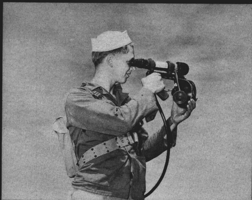
Official U. S. Navy photographs THE SNOOPERSCOPE has a dual mechanism: a light source which sends out infra-red rays to illuminate the target and a receiver to spot the target.
