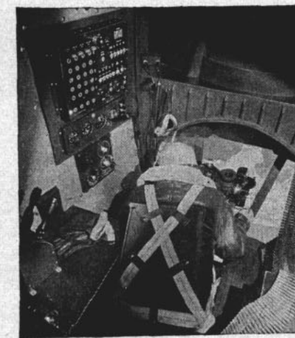
LIGHT-BEAM "BOMBS" are dropped by trainee in horizontal bomber trainer chamber which simulates actual conditions during flight.
