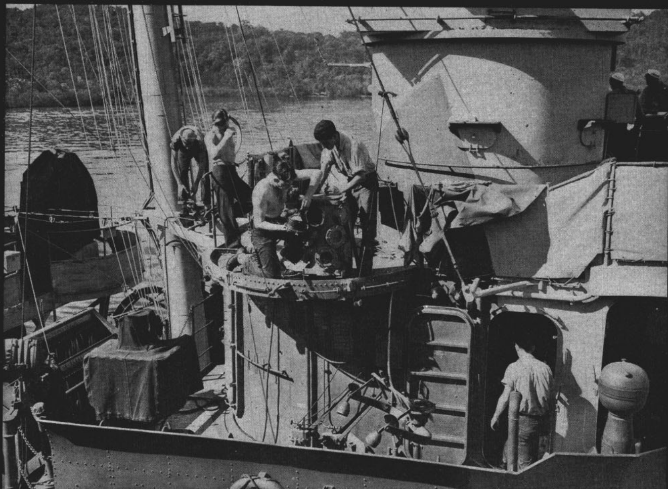
INFRA-RED UNIT is installed in a beacon, used during the war to send simultaneous messages to ships in formation.
