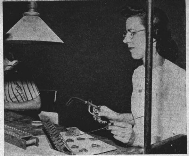
PURPLE HEARTS are smoothed (left) to a satin finish on rotating sanding strips. At right, holding rings are soldered on medals to decorate the Navy's most deserved by one of the many technicians at the Philadelphia mint.
