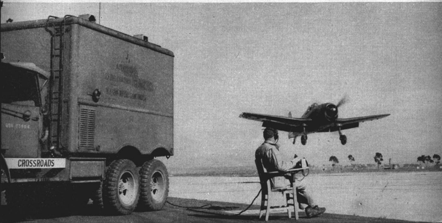
INTERCEPTION PROBLEM (above) concerns release of drone from one queen to other. Below, drone comes in for landing controlled by ground officer.
