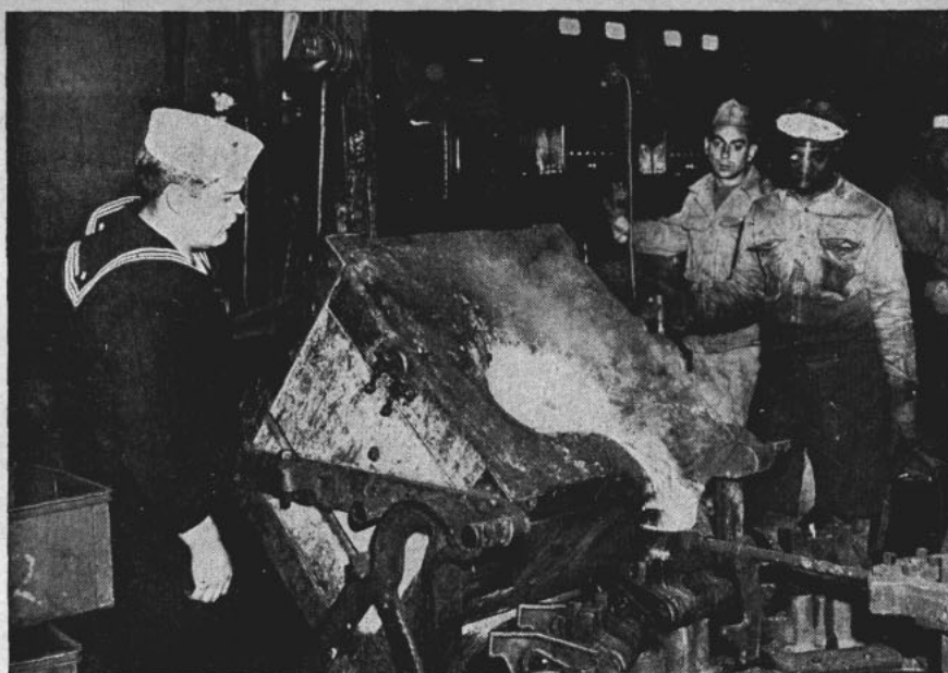
ELECTRIC FURNACE (left) in melting room of Philadelphia mint pours molten metal which eventually becomes Navy medals. At right, original galvano plates and plaster paris casts are shown to a Marine, injured on Okinawa.
