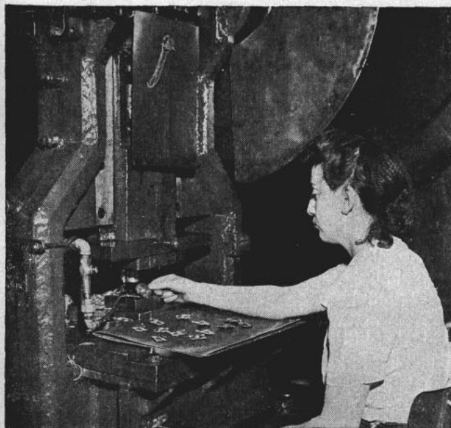
STAMPING OUT Navy Crosses (left) by applying 100 to 600 tons of pressure. Medals are restruck until figures stand out sharply in relief. At right, medals are examined closely for sharpness of design under magnifying lens.
