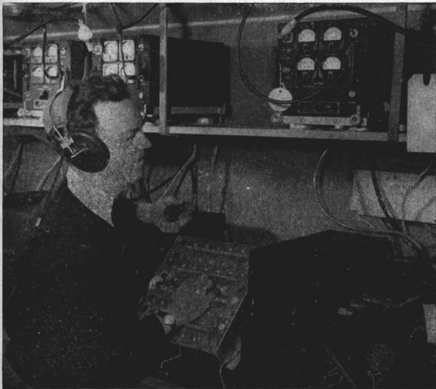
AVIATION RADIOMAN , working inside control booth, throws control switch to put ground officer's controls on same frequency as incoming drone plane.
