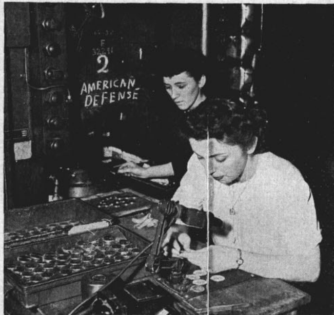
STAMPING OUT Navy Crosses (left) by applying 100 to 600 tons of pressure. Medals are restruck until figures stand out sharply in relief. At right, medals are examined closely for sharpness of design under magnifying lens.
