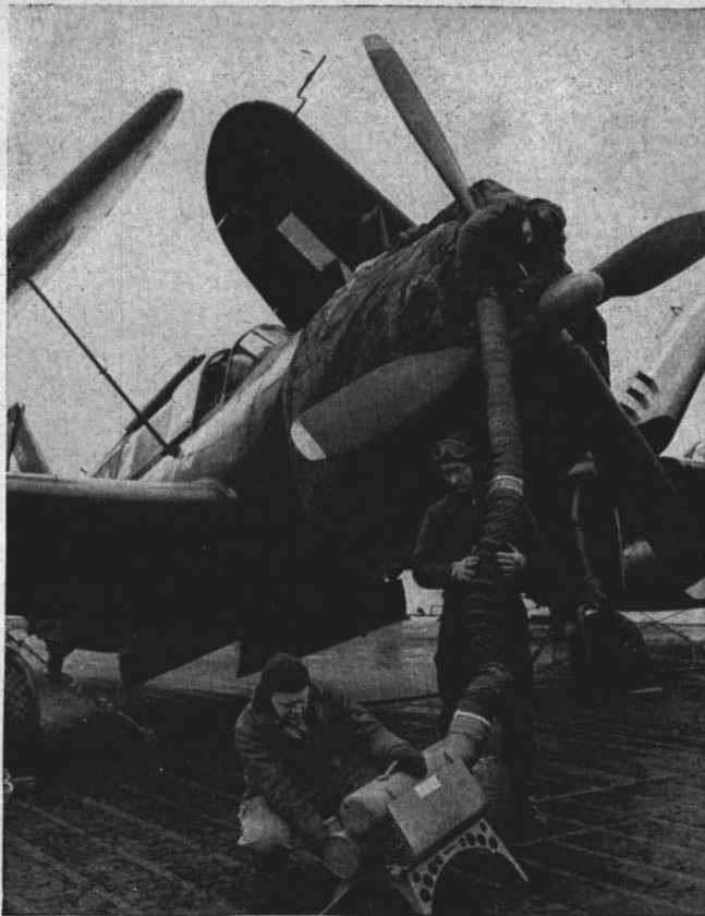
Official U. S. Navy photograph HOT AIR from a pre-heater is piped over the jacketed engine of a Helldiver in test of cold-weather equipment.
