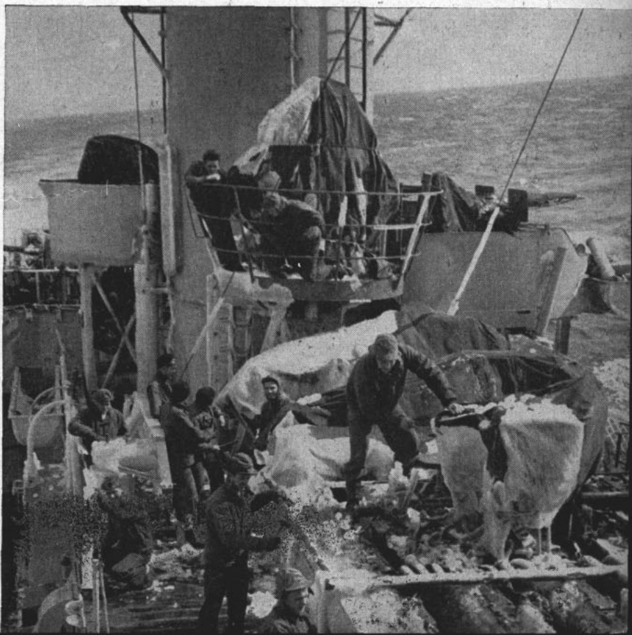
ICE COATING on torpedo tubes is removed by crew members of the destroyer USS Ware , member of Midway task group in "Operation Iceberg." Acme Photo
