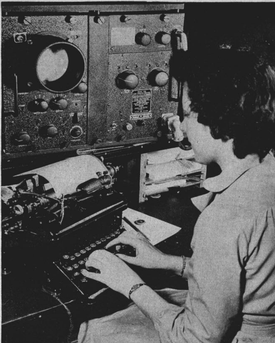
Official U. S. Coast Guard photograph RECEIVER INDICATOR , identical to those used on board ships for taking time difference readings, is shown in use at a shore-based monitoring station.
