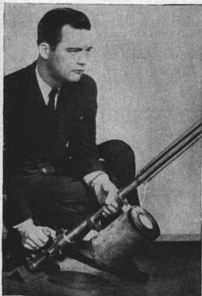
Official U. S. Coast Guard photograph A NEW LINE throwing gun perfected by James E. Seig, CGM, of the Coast Guard is said to have greater range than any previous line gun.
