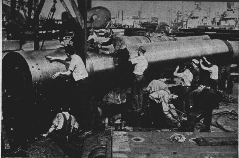
A SIXTEEN INCH rifle barrel receives its final polish by civilian workers at New York Navy Yard before installation in the USS Iowa main battery.
