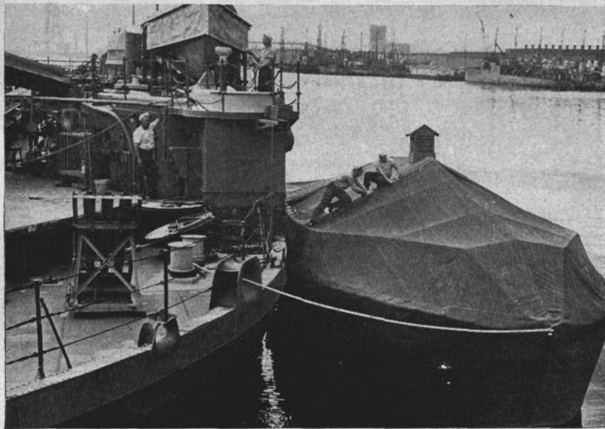
PT POSTWAR HOME may be under a canvas cover, as shown above, or in a sealed wooden shed ashore. Vital parts will be given protective coatings.
