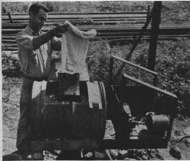
IMPROVEMENT over windmill and hand washers are motor-powered ones (above and at right). One above has a Jap motor. Blowtorch under drum heats the water.
