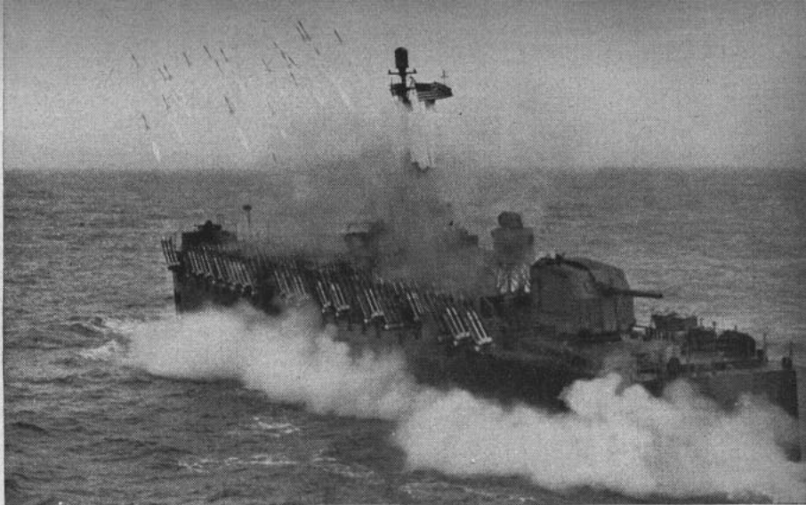
Official U. S. Navy photographs LIGHT AND MOBILE , but packing a terrific punch, rockets played a major role in the war. Above is a Navy LSM(R), Landing Ship Medium (Rocket)
