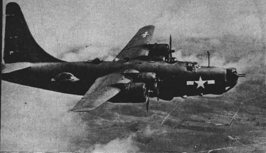
NEWEST Navy plane to be released in photograph is the Privateer, an Army Liberator redesigned for the Navy's long-range Pacific operations. The changes most apparent are the single tail assembly and gun blisters.
