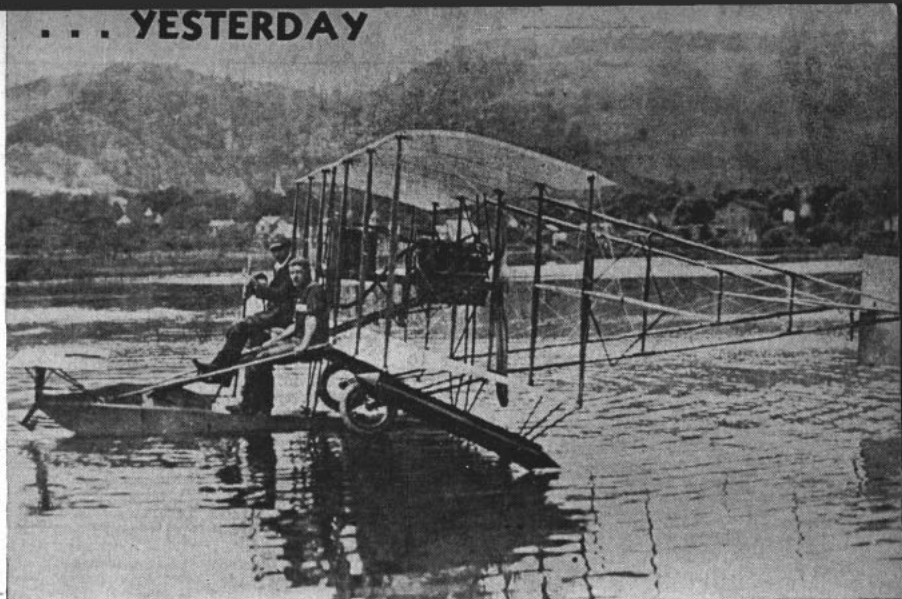
FIRST Navy plane was this Curtiss biplane, a jalopy in contrast to the giant Privateer opposite. The pontoon was the Navy's contribution to aircraft. This plane also had wheels, making it the first amphibian.
