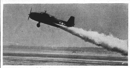
Avenger springs aloft with assistance of four 330-horsepower jet units.
