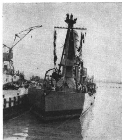
2 A temporary false bow was fitted to the SHAW after salvage. Then she reached Mare Island.
