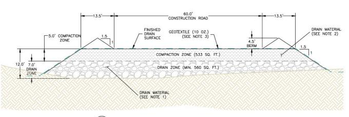
D FLOW-THROUGH DRAIN TO PWTS POND AREA - TYPICAL SECTION SCALE: 1"= 10' (22"x34" FORMAT)
