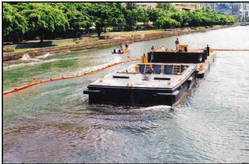
Photo 3. Push boat transporting dredging equipment. Source: American Marine Corp., 2002-03
