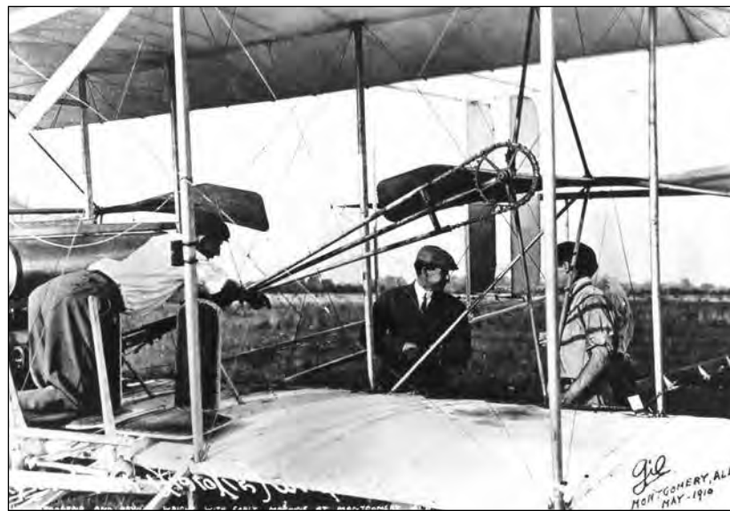
(Above) Spencer Crane, one of the student aviators at the Wrights' school, checks one of the propeller transmission chains. With no automated lubricating system, the chain drive system had to be lubricated at regular intervals.
