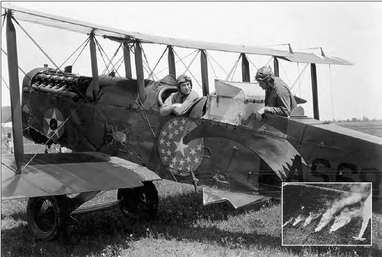
Two-man crew on a plane from Maxwell Field, fitted with a hopper and chute for dispensing pesticide. Note the boll weevil depicted on the fuselage. A series of aircraft disperses pesticides in test runs conducted by pilots from Maxwell Field in collaboration with the US Department of Agriculture Research Lab and Huff-Daland Dusters ( inset ; photo courtesy of Delta Airlines).
