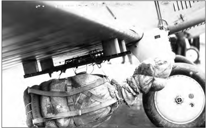
An outboard motor wrapped in a tarpaulin loaded underneath a Maxwell Field aircraft for delivery to southern Alabama
