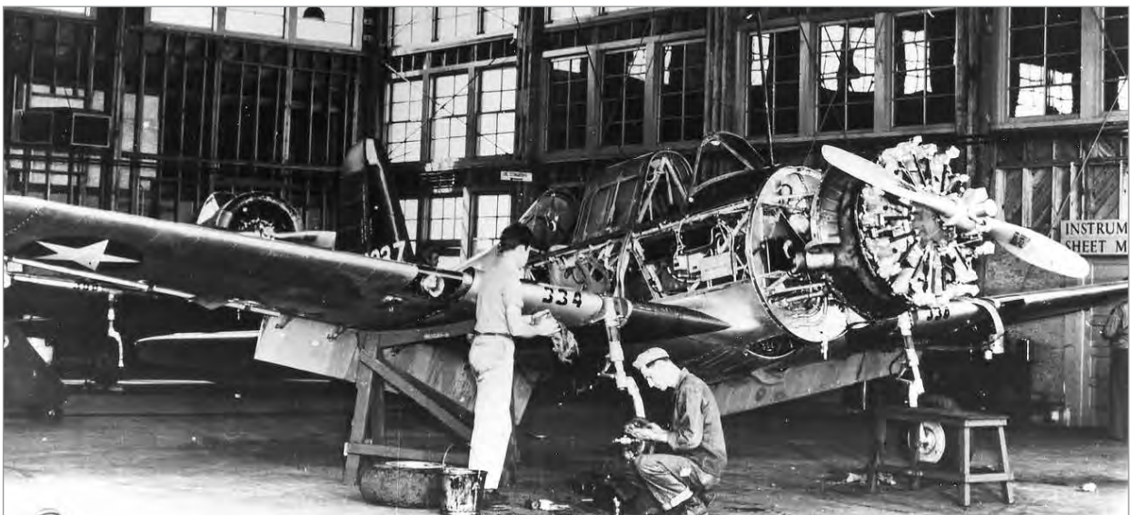
A BT-13 undergoing an engine overhaul in a Gunter Field hangar
