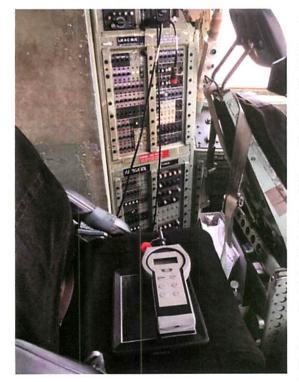
Figure 14 - 165 AW Precision Tachometer Plugged into WC-130H T/N 65-0984 (Tab Z-8)
