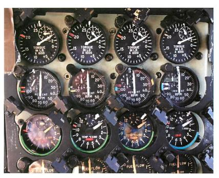
Figure 15 - WC-130H T/N 65-0984 Engine Performance Gauges (Torque, RPM, and Temperature) (Tab Z-13)
