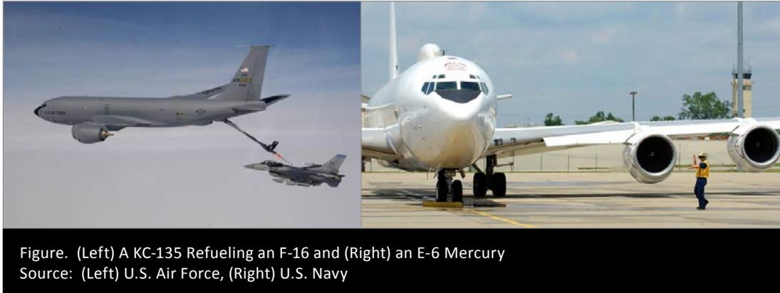
Figure. (Left) A KC-135 Refueling an F-16 and (Right) an E-6 Mercury
