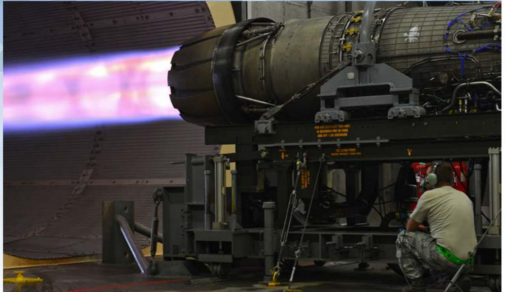
An aerospace propulsion craftsman examines an afterburner during an F-16CM Fighting Falcon engine check. The new ISWAT technology accounts for this type of maintenance during wargames. Previously, aircraft were only removed from simulations if destroyed in combat. (U.S. Air Force photo/Airman 1st Class Christopher Maldonado)
