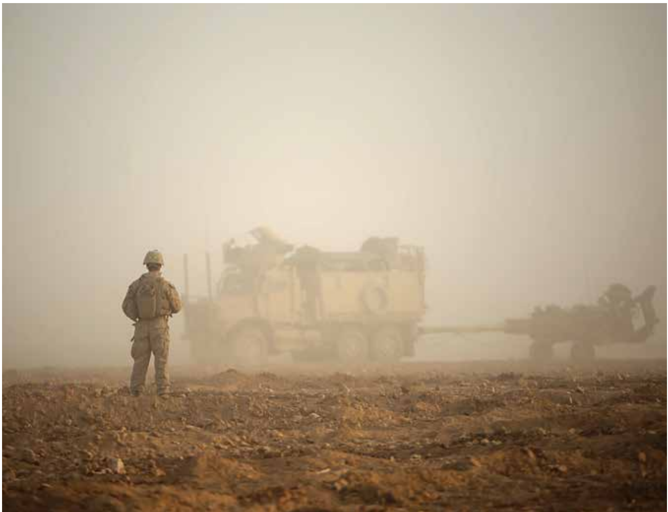
A U.S. Marine waits to guide a troop movement armored vehicle (TMAV) towing an M777-A2 Howitzer to a firing position in Syria. (U.S. Marine Corps photo)
