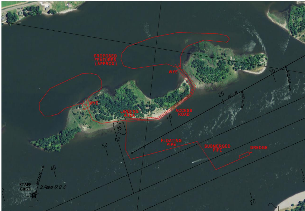
Figure 8 Dredging elements (landing, access road, pipe, wye, etc.)
