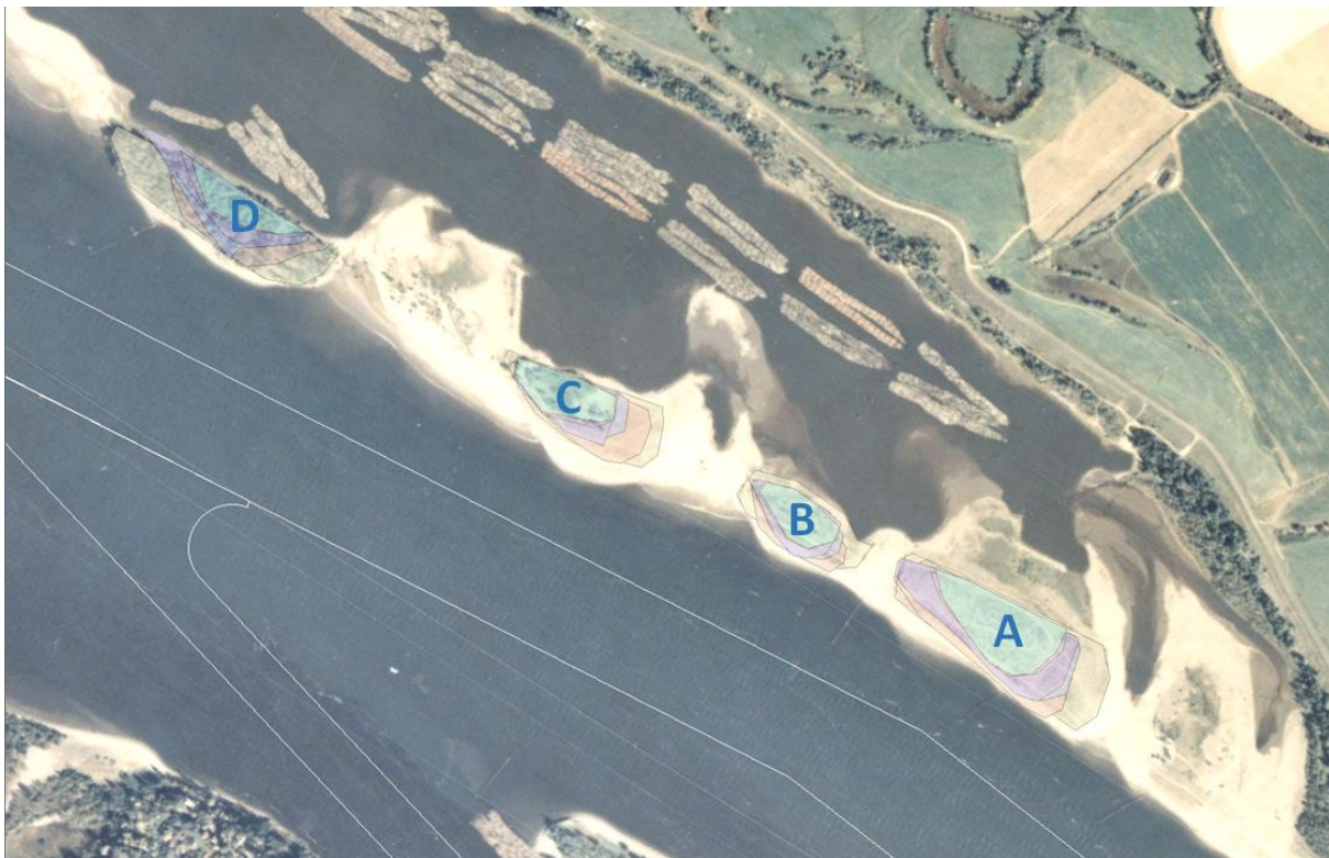
Figure 2.17. Estimated aerial extents of land above ordinary high water (OHW) overlaid on 1977 imagery.
