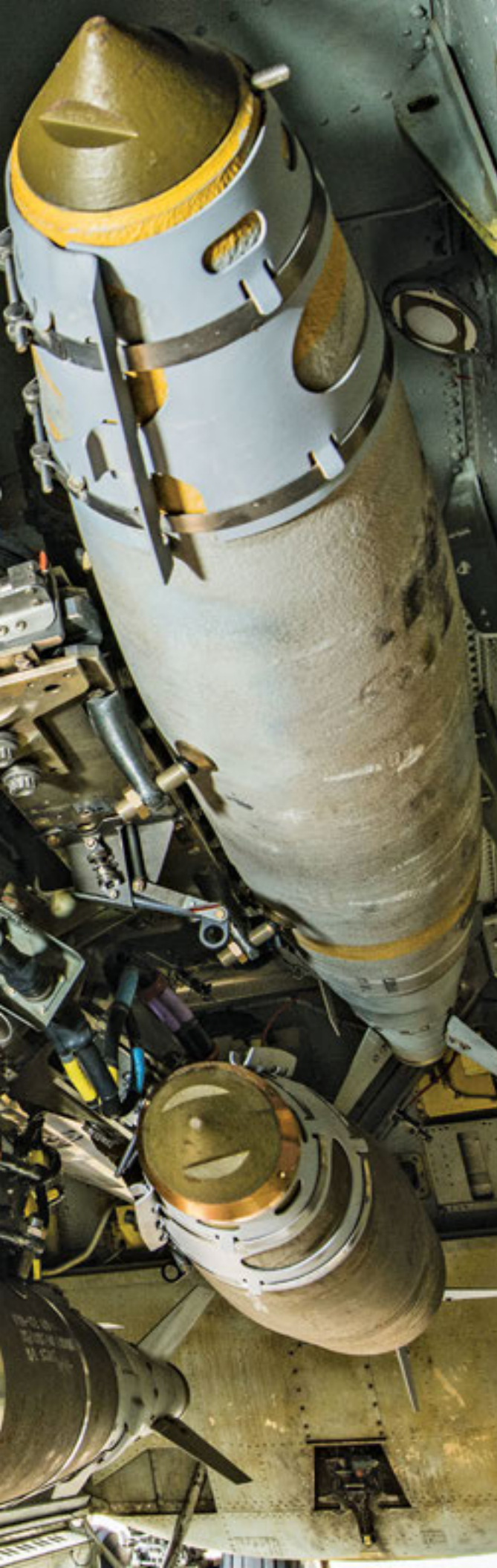
A U.S. B-52 Bomber sits on a flightline with munitions loaded on a newly installed conventional rotary launcher in its bomb bay. (U.S. Air National Guard photo)
