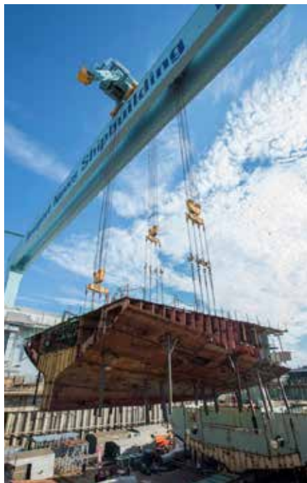
Above and right: Newport News Shipbuilders lifted a 704-metric-ton unit into Dry Dock 12, where construction of the aircraft carrier USS John F. Kennedy (CVN-79) is taking shape. —photo by Chris Oxley, Huntington Ingalls Industries
