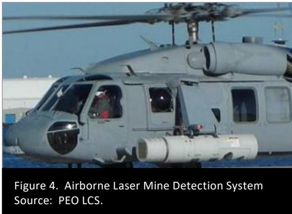
Figure 4. Airborne Laser Mine Detection System
