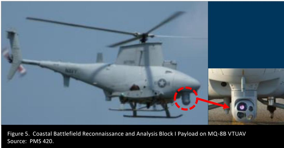
Figure 5. Coastal Battlefield Reconnaissance and Analysis Block I Payload on MQ-8B VTUAV
