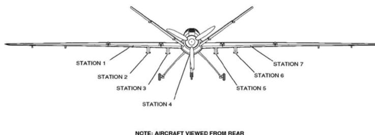
**Figure 3. MQ-9 station depiction.** (Reprinted from TO 1Q-9(M) A-34-1-1, *Technical Manual, USAF Series MQ-9 Aircraft Nonnuclear Munitions Delivery*, change 1, 1 March 2014, 1-3.)
