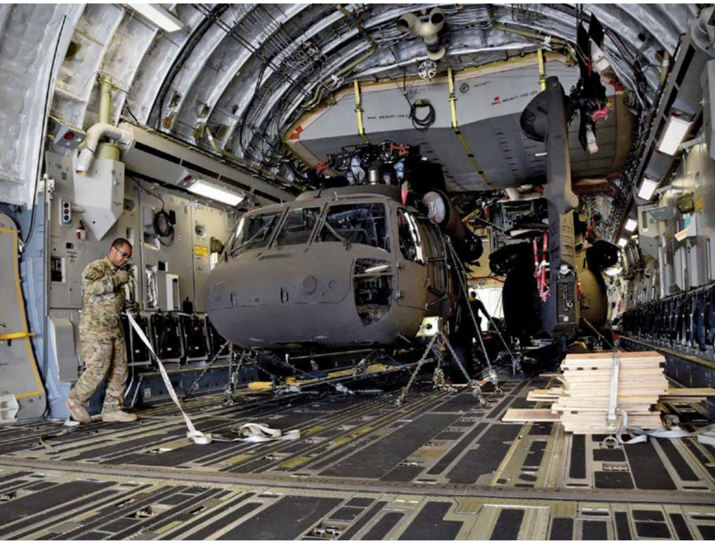
A U.S. Air Force C-17 loadmaster prepares two Afghan Air Force UH-60 helicopters for unloading at Kandahar Air Field. (U.S. Air Force photo)
