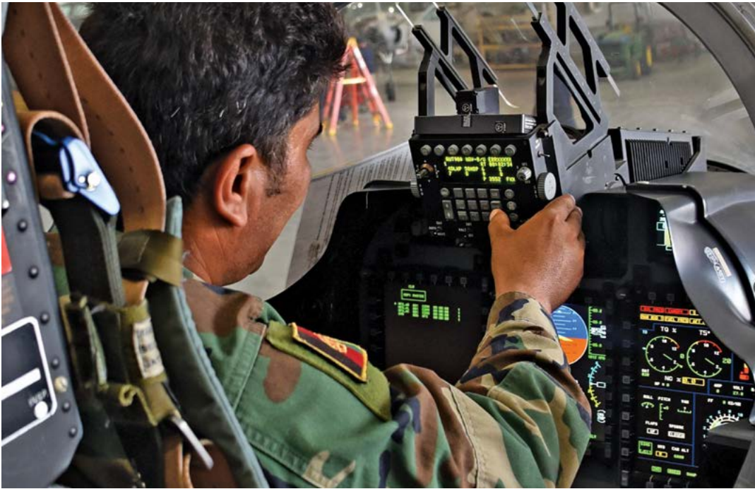
An Afghan Air Force A-29 Super Tucano maintainer performs an avionics check in the cockpit of the aircraft at Kabul Air Wing. (U.S. Air Force photo)
