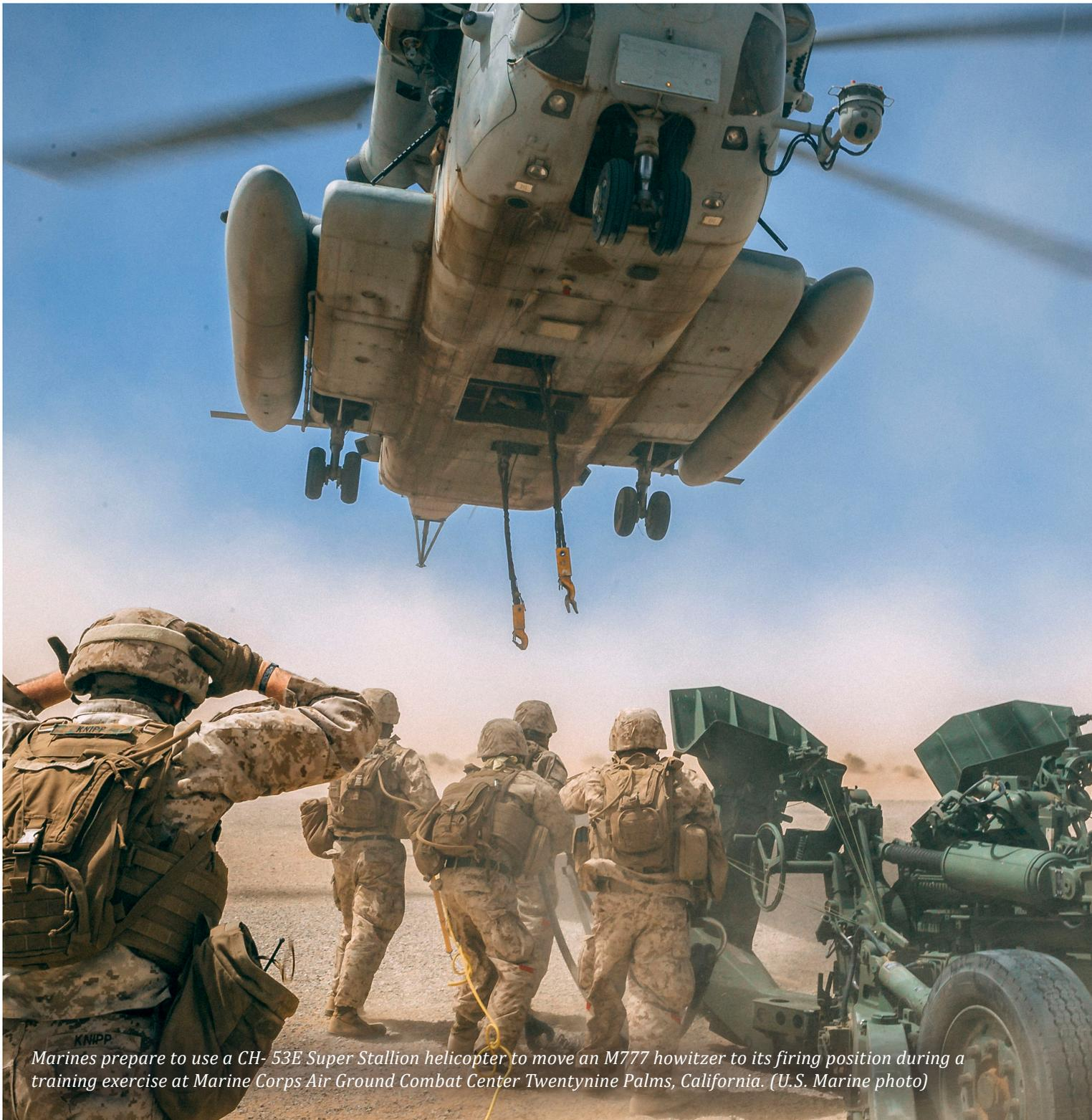
*Marines prepare to use a CH-53E Super Stallion helicopter to move an M777 howitzer to its firing position during a training exercise at Marine Corps Air Ground Combat Center Twentynine Palms, California. (U.S. Marine photo)*
