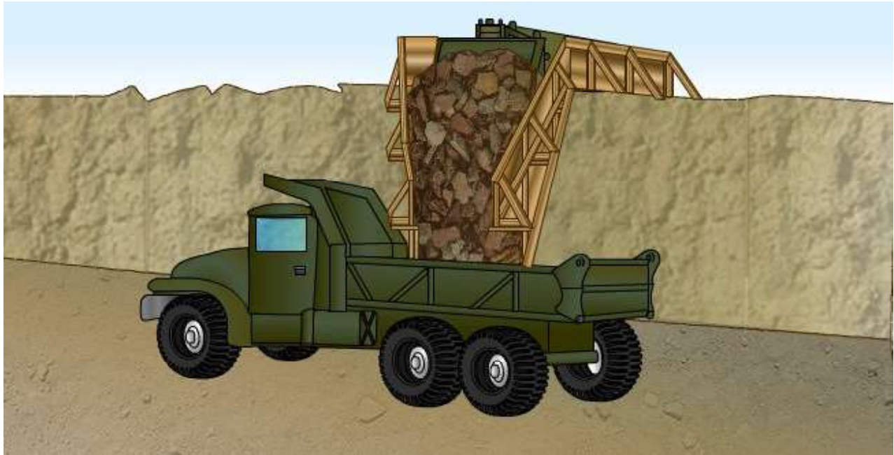
Figure 5-8 – Plain chute loading ramp.
