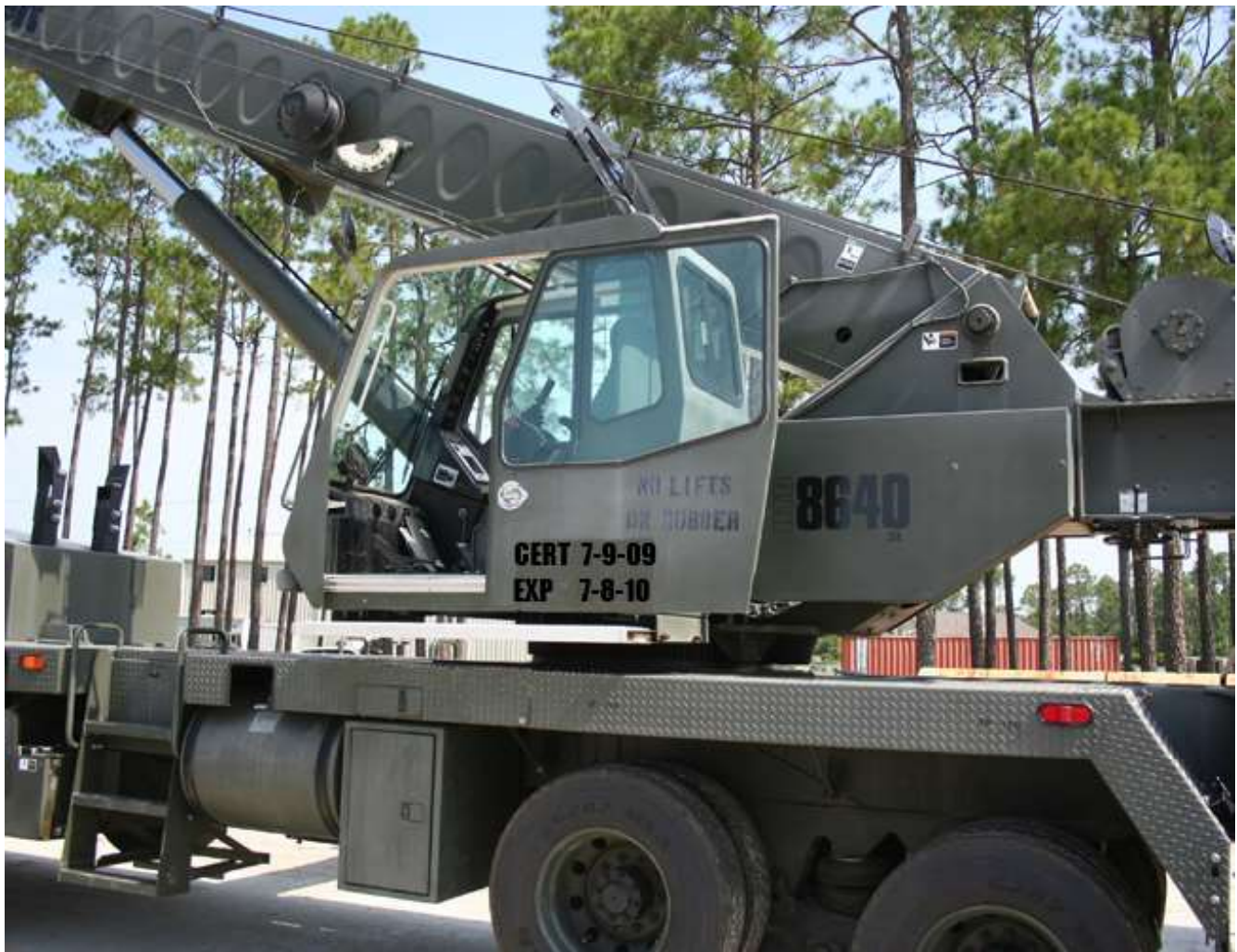
Figure 3-12 – Date of certification on crane.
