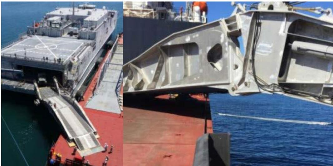
Figure 2. EPF Stern Ramp and Mobile Landing Platform Used for At-Sea Transfers.
