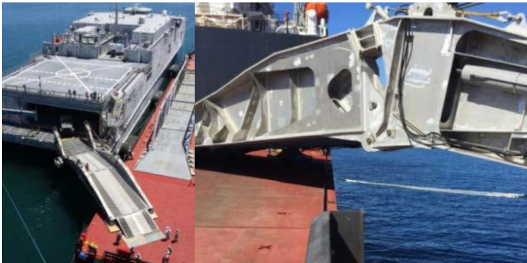
Figure 2. EPF Stern Ramp and Mobile Landing Platform Used for At-Sea Transfers. Source: COMOPTEVFOR FOT&E Report.
