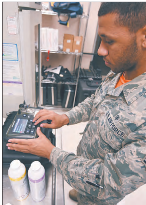
U.S. AIR FORCE PHOTO BY SENIOR AIRMAN HARRY BREXEL U.S. Air Force Senior Airman Emery Coleman, 19th Aerospace Medicine Squadron bioenvironmental engineering technician, uses a Hazardous Material Identification System to check a soil sample for contaminations March 24 at Little Rock Air Force Base. Bioenvironmental engineering technicians respond to terrorist attacks, natural disasters and accidents to identify potential health hazards.
