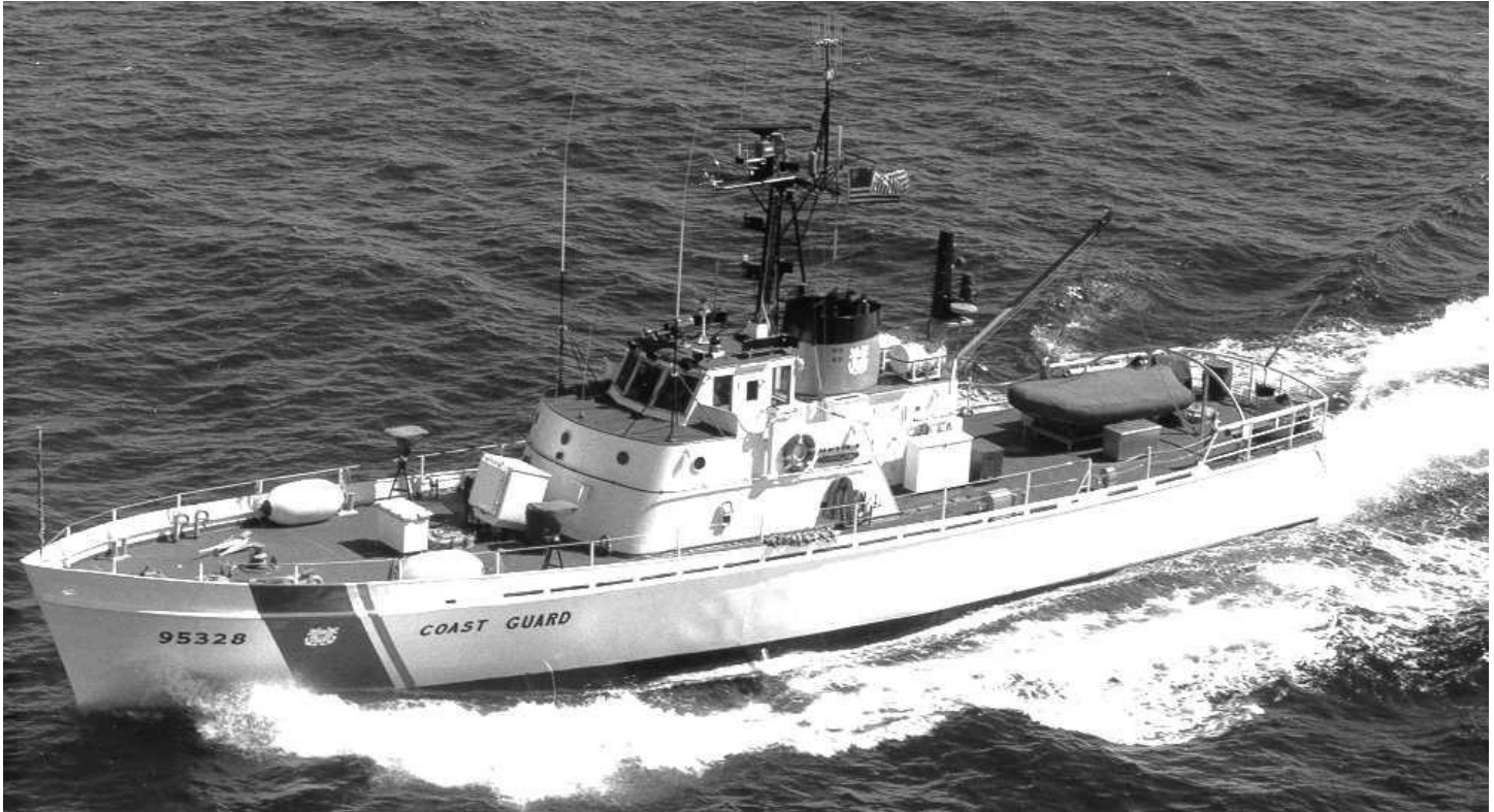
WPB-97328 Cape Henlopen underway circa 1990. Armament reduced to mounts of 50-cal. m.g. A member of the "C" class, my guess is that she has received the renovations mentioned above.
