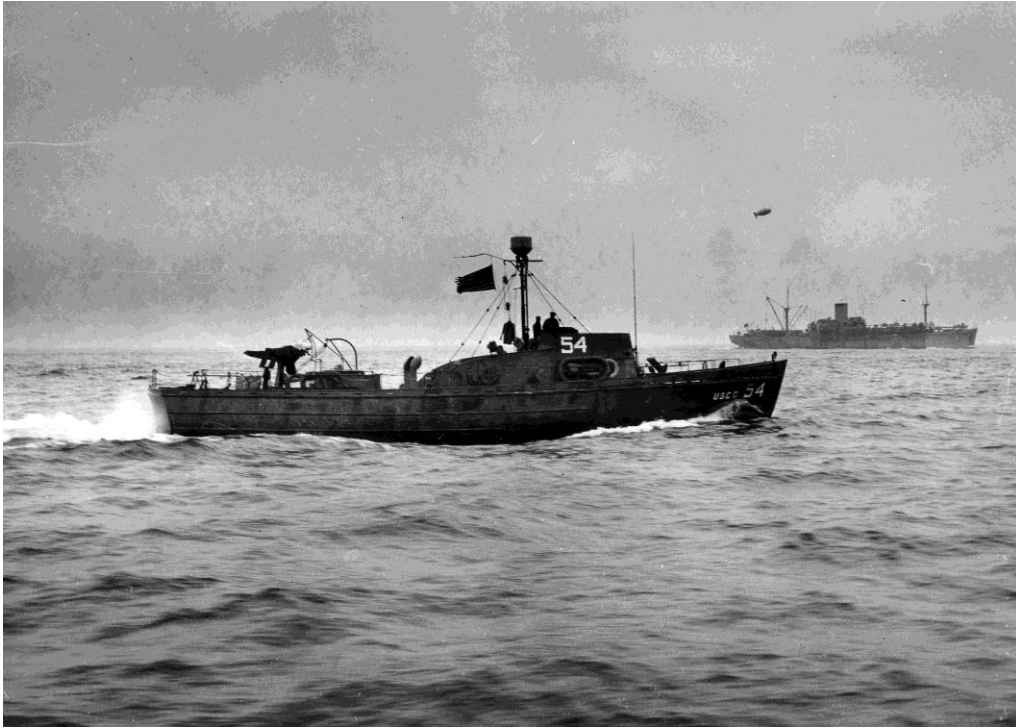
CG-54 (CG-83502) off Normandy June 1944. Note flat top of wooden wheel house.
