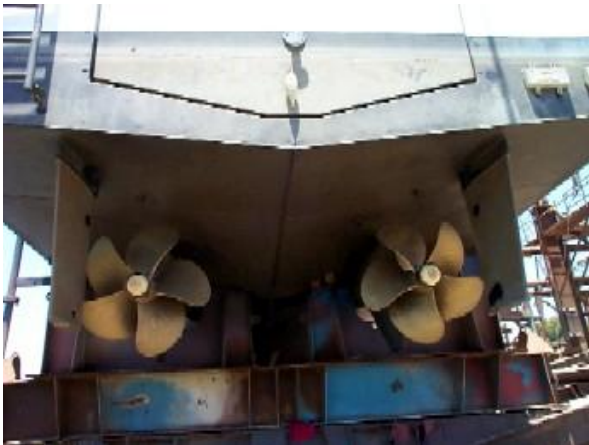
Haddock's stern showing 5-bladed props
