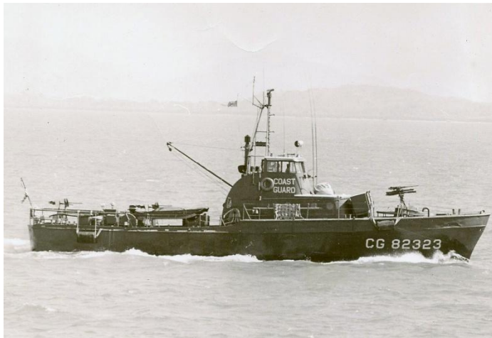
Two sisters from Squadron One in Viet Nam War Paint WPB-82323 Point Grace and 82327 Point Banks circa 1968. Both mount the usual over-under 50-cal m.g. and 81-mm mortar combo in the bow, while additional 50's are mounted aft.
