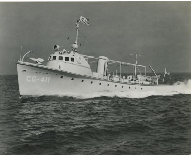
The CG-411 is an 80-footer and can make 26 knots.
