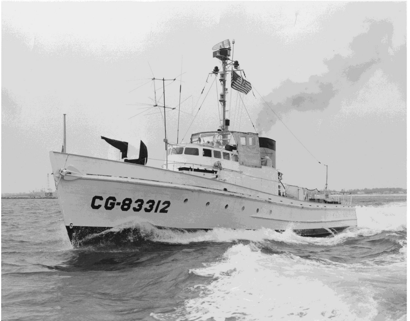
Another later view of CG-83312 27 Apr 1959. Note updated radar, TV antennae, and 20-mm gun forward. It also appears that she has been fitted with diesels engines and thus the stack which has been added aft of the wheel house.
