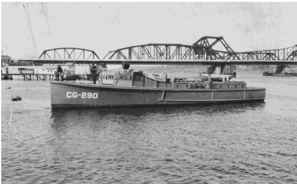
CG-290 with top works modified. It appears her mast was removed to allow her to fit under bridges like the one in the background.
