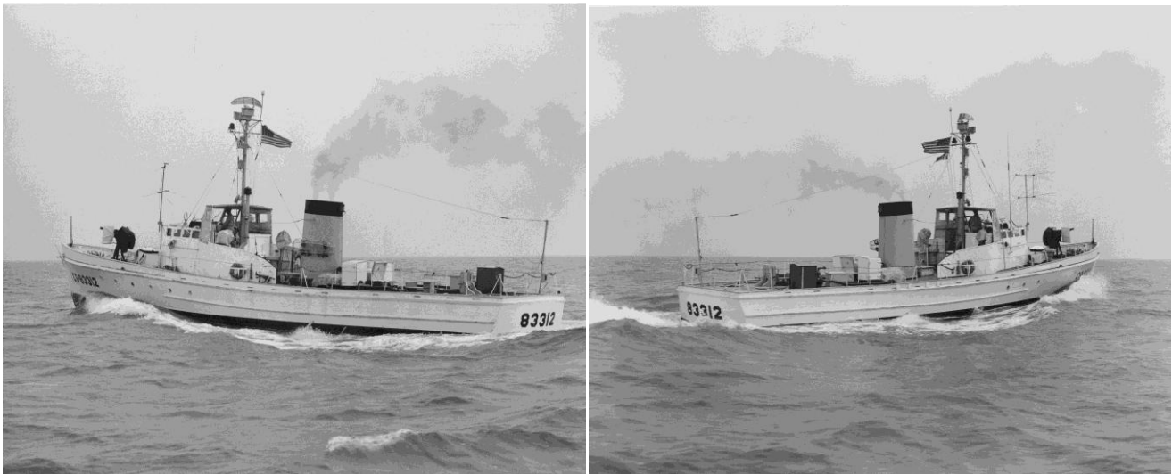
Two more views of the CG-83312 showing the stack to better advantage. Smoke appears to be diesel exhaust.
