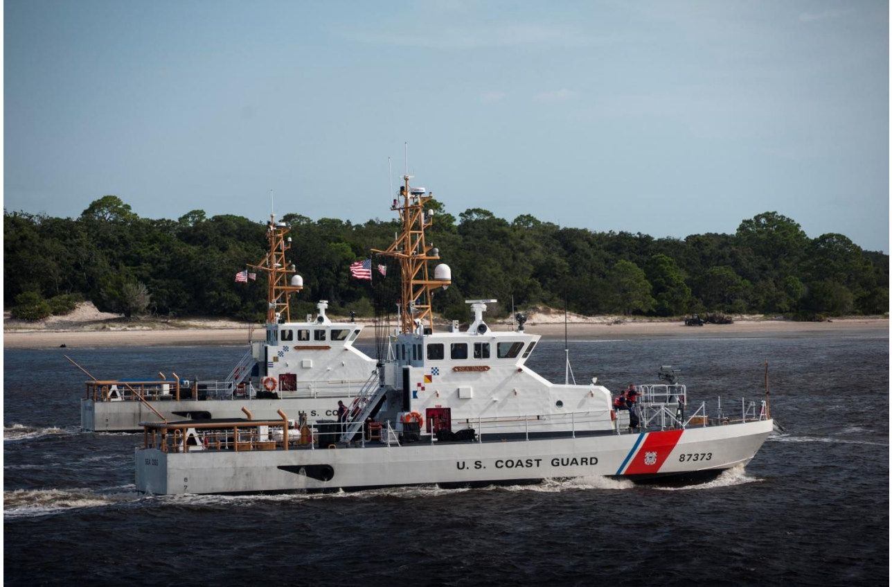
WPB-87373 Sea Dog and WPB-87367 Sea Dragon off Kings Bay, GA. Note raised, remotely operated gun mount forward.
