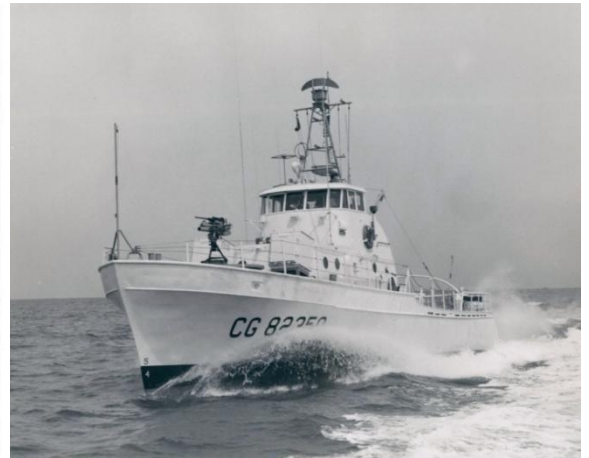
WPB-82340 Pt. Batan & 95320 Cape Starr fight barge fire in 1980's. WPB-87350 Pt Franklin circa 1963 with over-under m.g. & 81-mm mortar forward.
