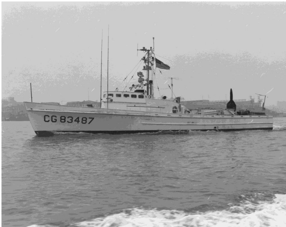
CG-83487 underway circa 1958, note 20-mm aft, and TV Antenna aft of wheelhouse.
