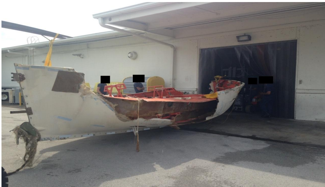
Figure 65. EL FARO Starboard Lifeboat. Heavy damage to the starboard side of the lifeboat is visible. Photo taken at Coast Guard Air Station Miami.
