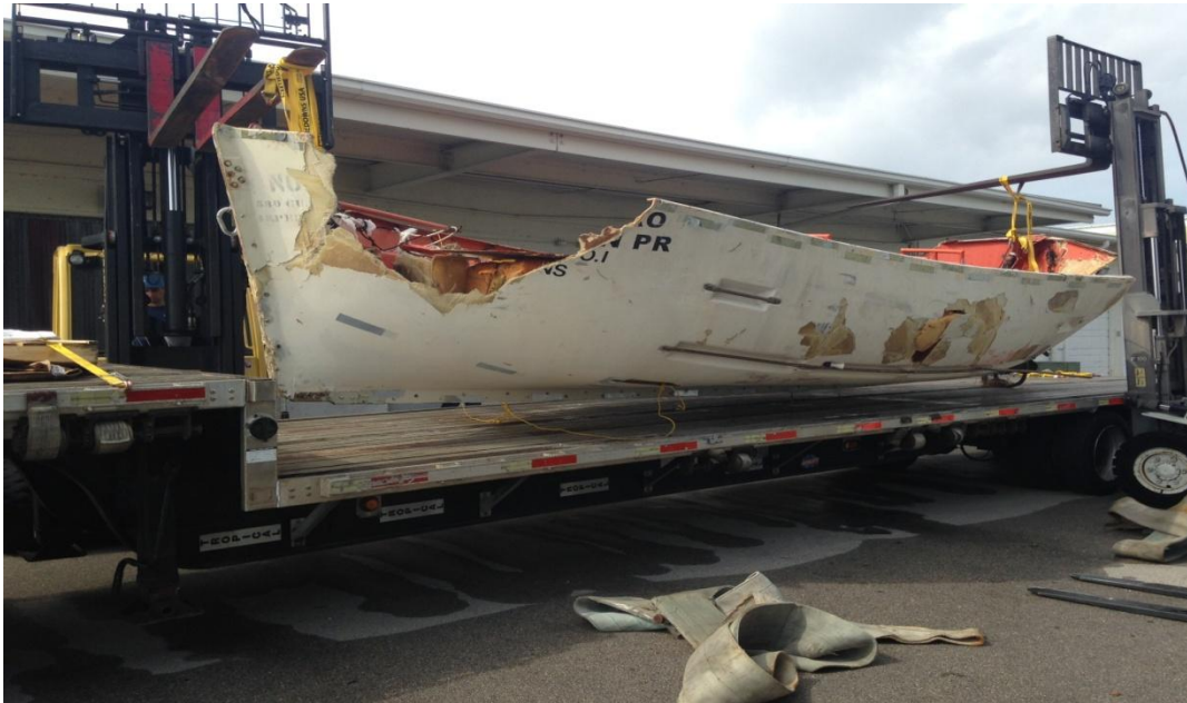
Figure 66. EL FARO Starboard Lifeboat. Damage to the port bow of the lifeboat is visible. Photo taken at Coast Guard Air Station Miami.
