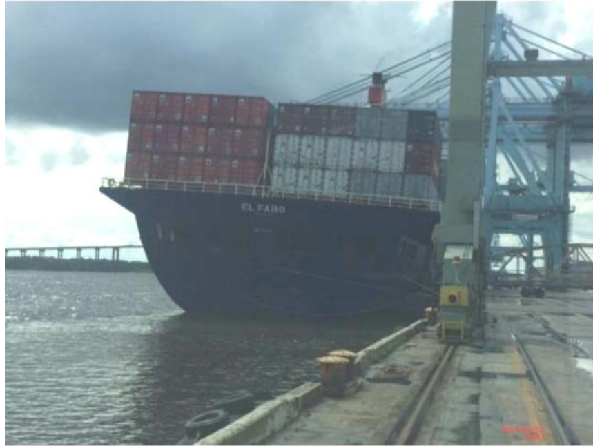
Figure 3. Photograph taken by TMPR Terminal Manager on September 29, 2015, showing starboard list of approximately 4 degrees during loading operations prior to the final voyage.
