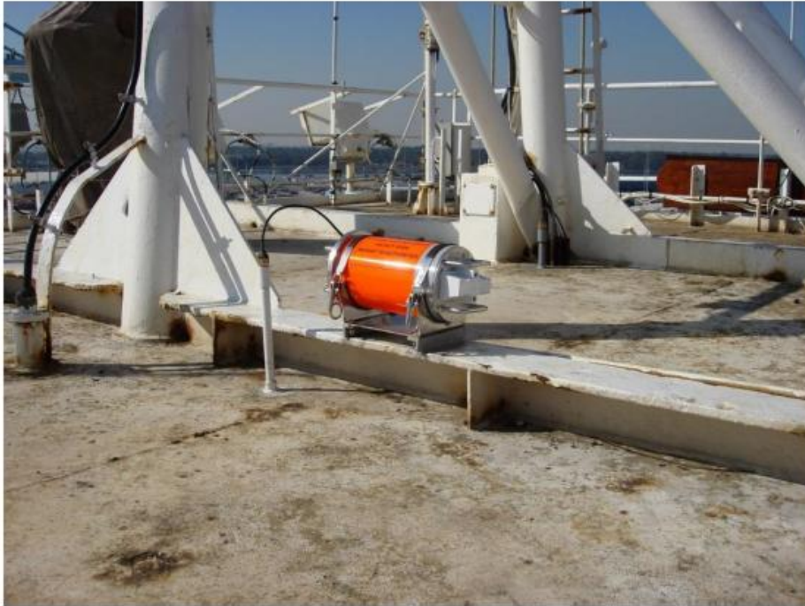
Figure 62. Archive photo of the EL FARO S-VDR capsule mounted on a beam on the flying bridge, port side. (Source: Radio Holland)
