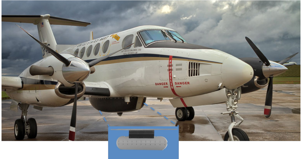
A Navy RC-12 King Air with an Applied Signals Intelligence payload attached. This version uses the direction finder functionality developed under the Air Force SBIR Program to take unique spectrum measurements for the Office of Naval Research. (Courtesy photo)
