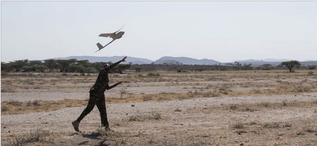
Figure 5. Kenyan Defense Forces Soldier Launches Raven Unmanned Aerial Vehicle (UAV) Source: Defense Video and Imagery Distribution System.
