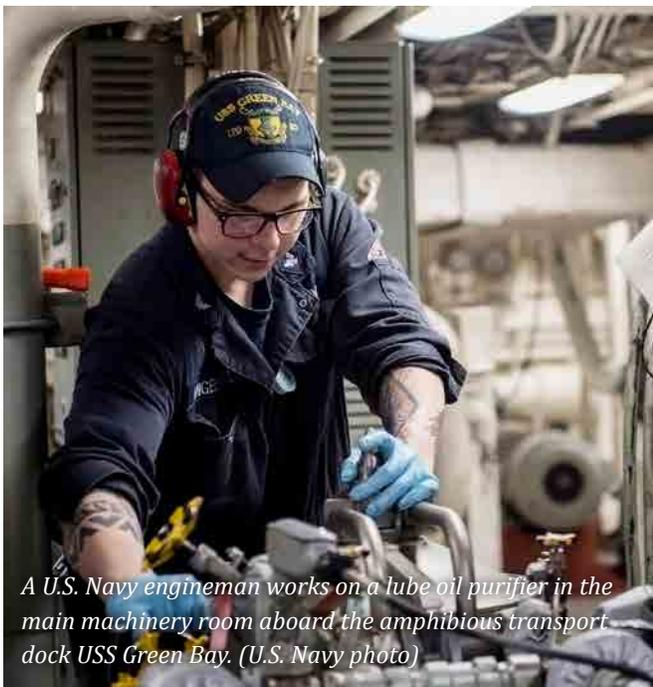
*A U.S. Navy engine room technician works on a lube oil purifier in the main machinery room aboard the amphibious transport dock USS Green Bay. (U.S. Navy photo)*
