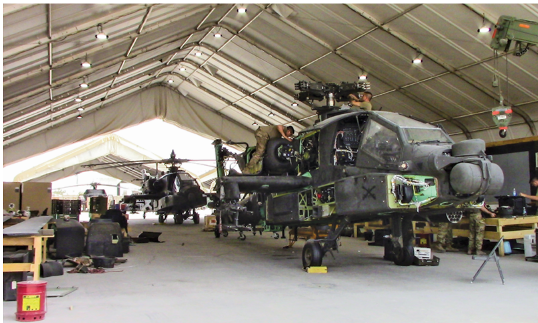
500-hour phase maintenance cycle of the AH-64E Apache “Guardian” at Camp Taji Military Complex, Iraq. (U.S. Army photo)
