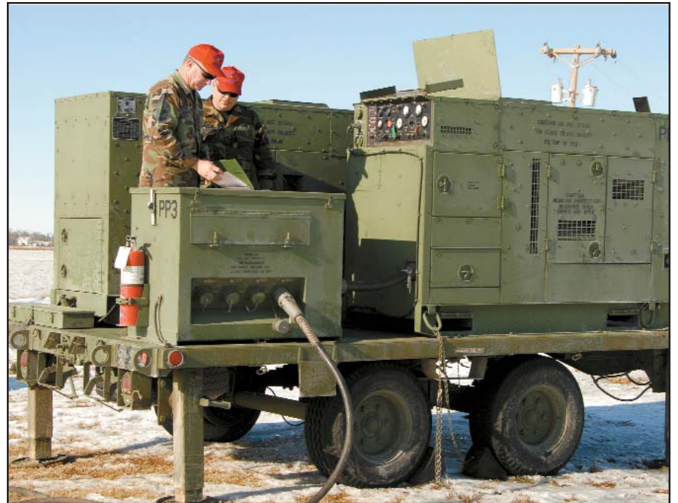
Senior Master Sgt. Bill Angstadt and Tech. Sgt. Keith Woodrome from the 134th Air Control Squadron, 184th Air Refueling Wing, operate a power generator in Utica, Kan. This generator is providing power to a water pump station that supplies water to Utica and surrounding communities. (Photo by Capt. Debbie Balentine)
