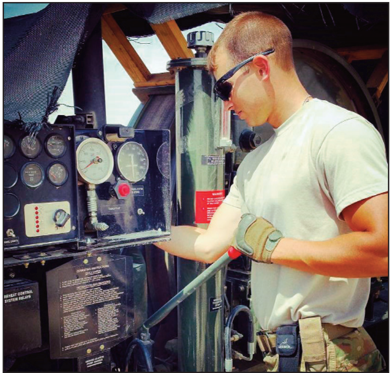
An airman from the 184th Civil Engineering Squadron performs maintenance on an Aircraft Arresting System while deployed to an undisclosed location in Southwest Asia.
