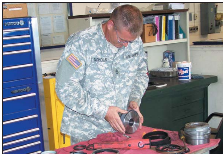
Staff Sgt. Anthony Nichols repairs internal components while rebuilding a hydraulic cylinder from a M10A forklift.
