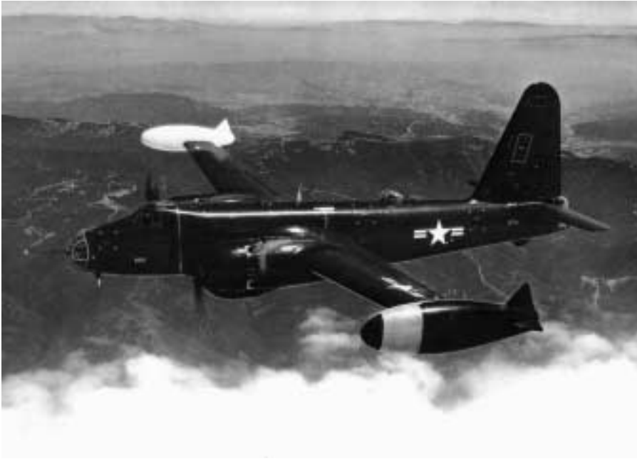
Modified Navy P2V Neptune patrol planes conducted electronic reconnaissance missions along the coast of China and the Soviet Far East during the Korean War.
