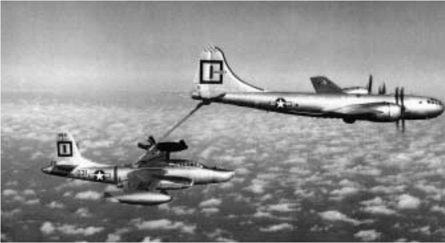
A Boeing KB-29P extends the 1,910 NM-maximum range of a North American RB-45C Tornado by aerial refueling.
