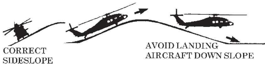
Figure 4-3. Determining Ground Slope
