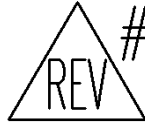
FIGURE 7: REVISION TRIANGLE BLOCK (REVTRIBLK) NOTE: Revision triangle used to show where change was required.
