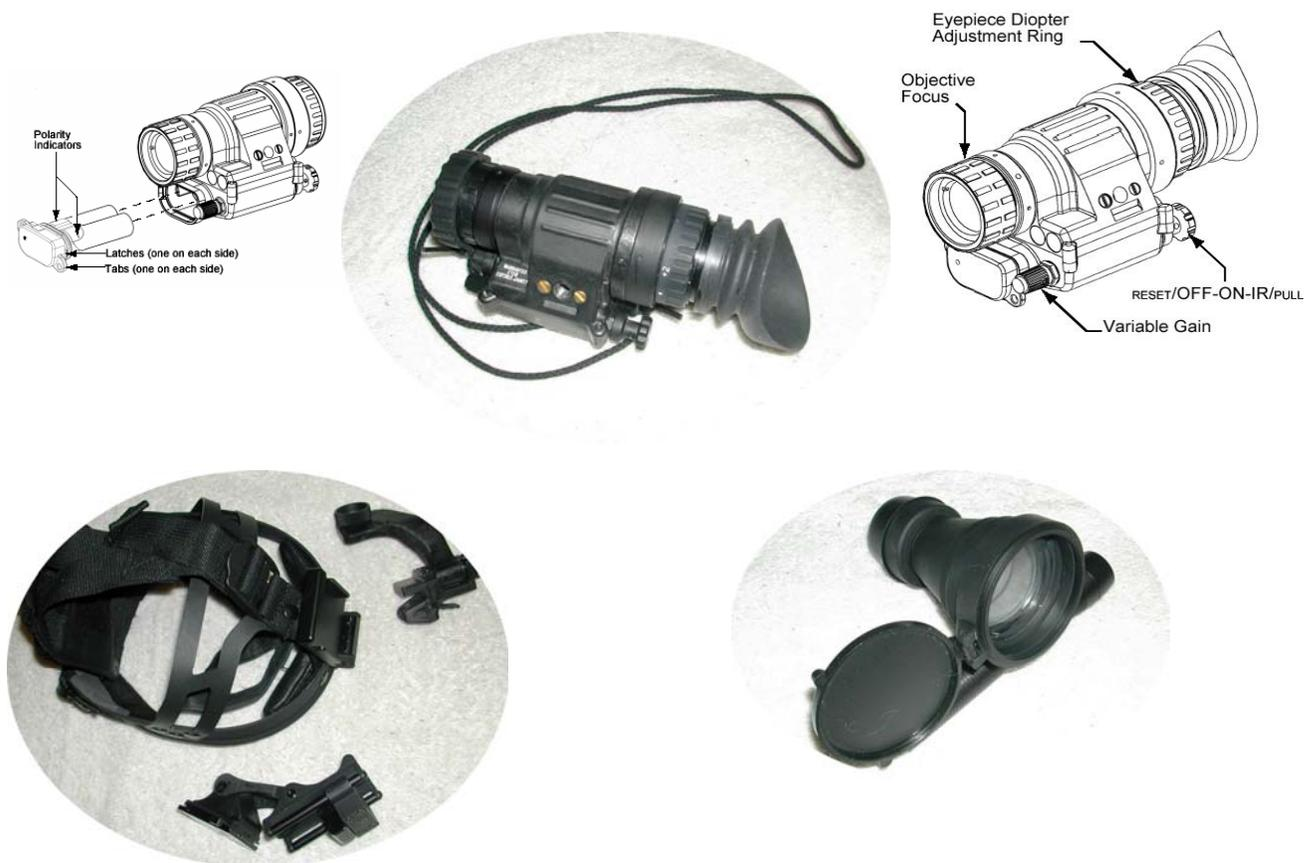
Night vision MNVDs are ruggedized and as a result, are very durable. With proper care and maintenance, they should last for many years. Use fresh water, **NO** chemicals to rinse away dirt and debris after use. Dry with a soft, lint-free cloth. Clean with a lens pen or lens paper. Store in a dry place.
