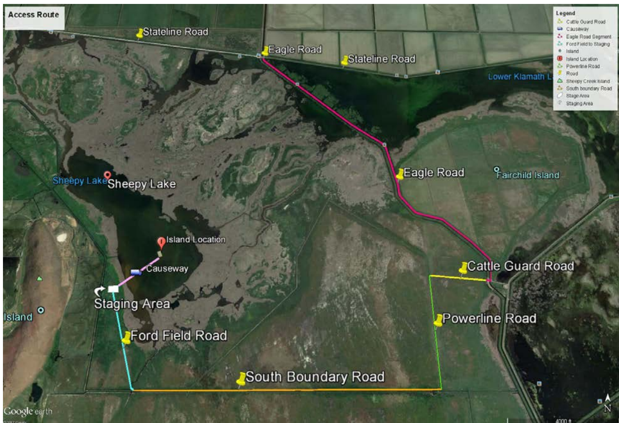
Figure 3.4 Location of proposed access route, staging area, temporary road and island location.
