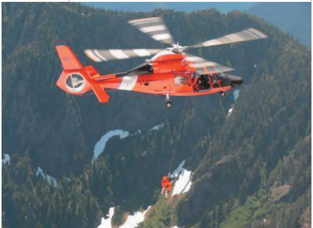
Fig. 4: A newly re-engined U.S. Coast Guard HH-65C DOLPHIN helicopter assigned to Coast Guard Air Station Port Angeles, Wash., rescued an injured hiker from a near-vertical mountain slope at an elevation of 6,300 feet in Washington State in July. The DEEPWATER Programme's conversion of older DOLPHINS to the more powerful HH-65C multi-mission helicopter made the difference in enabling the operation. Maritime safety, search, and rescue are some of the Coast Guard's best publicised responsibilities. On a typical day in 2005, Coast Guard fixed-wing aircraft, helicopters, cutters, and small boats saved 15 lives, assisted 117 people in distress, and conducted 90 search-and-rescue cases. (Photo: Courtesy U.S. Coast Guard)
