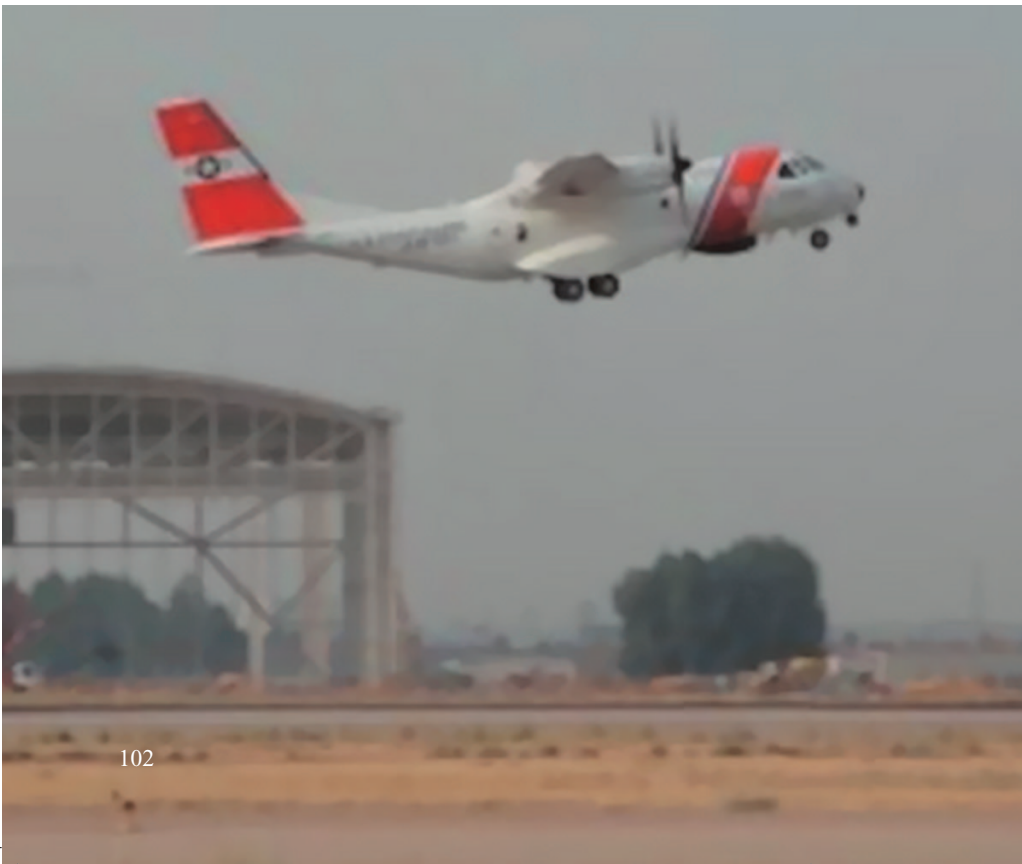
Fig. 6: The first EADS-CASA HC-235A medium-range maritime patrol aircraft was rolled out at its factory in March and made its first flight in June; it is shown here during a test flight at the EADS-CASA facility in Seville, Spain, piloted by a U.S. Coast Guard aviator. The DEEPWATER Programme also is upgrading the inventory of the Coast Guard's long-range search aircraft, including missionisation of six improved HC-130J aircraft. Small and medium-range helicopters also are being modernised and converted to serve as more capable multi-mission platforms as part of the DEEPWATER Programme. (Photo: Courtesy EADS-CASA)
